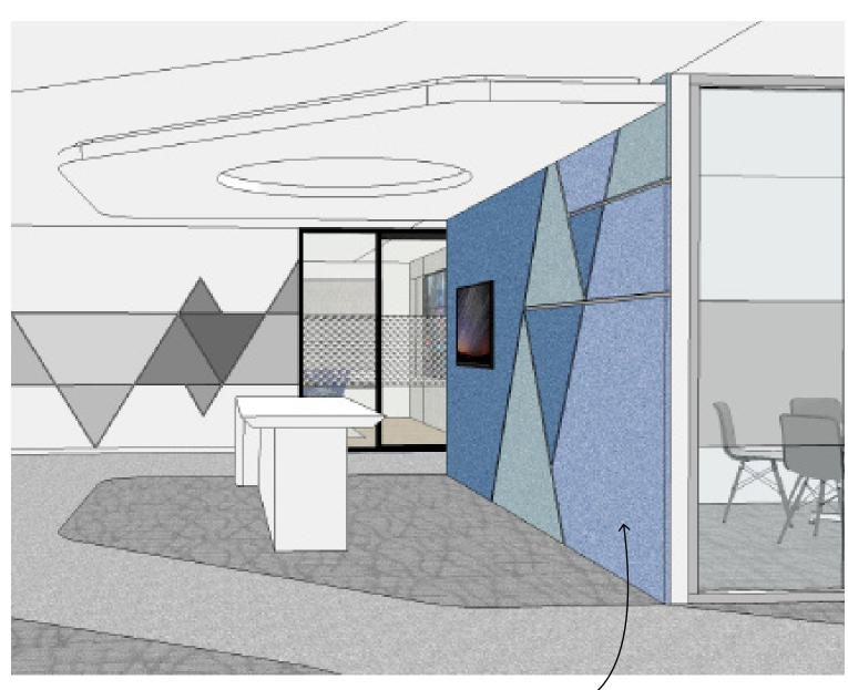
acoustic wall and acoustic soffit helps to dampen the sound generated from conversations in the open
